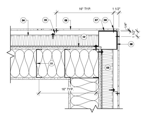
(01) ASSEMBLY OF A STEEL HALF-TIMBERED WALL ACCORDING TO THE ARCHITECT.
