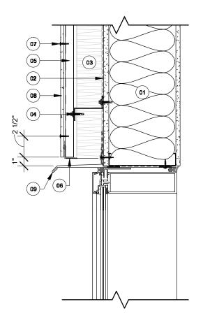
(01) ASSEMBLY OF A STEEL HALF-TIMBERED WALL ACCORDING TO THE ARCHITECT.
