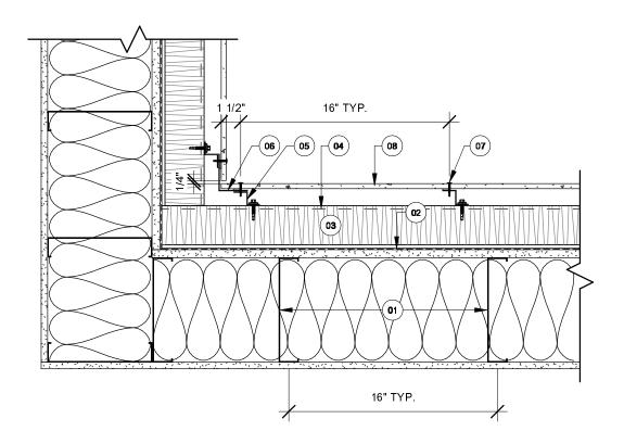
(01) ASSEMBLY OF A STEEL HALF-TIMBERED WALL ACCORDING TO THE ARCHITECT.
