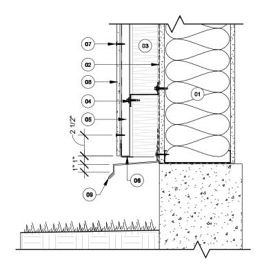
(01) ASSEMBLY OF A STEEL HALF-TIMBERED WALL ACCORDING TO THE ARCHITECT.
