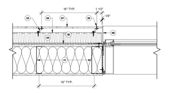
(01) ASSEMBLY OF A STEEL HALF-TIMBERED WALL ACCORDING TO THE ARCHITECT.
