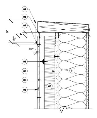
(01) ASSEMBLY OF A STEEL HALF-TIMBERED WALL ACCORDING TO THE ARCHITECT.
